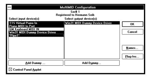
Use this dialog box to select the input and output driver(s) to be overlayed.
