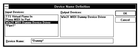
Here, all devices that are highlighted in the main configuration dialog's list boxes are displayed. If you select one of the devices, you can add an alias name in the edit field at the bottom of the dialog.
